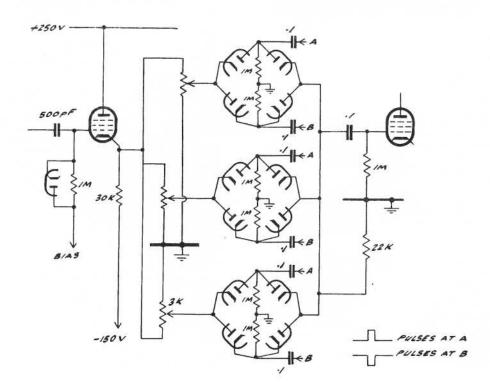
This is an improvement on the circuit shown in CQ-TV 21, it was found that the lift controls are not necessary with the C.P.S. Emitron. (An improved version of the Orthicon tube) A three tube self running multivibrator might be used instead of the ring counter (Electronic Engineering Feb. 1958), in this case it would be possible to synchronise it with a colour indexing pulse at one third frame frequency.
